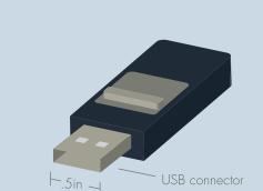
Container Rigid plastic shell encasing a USB
