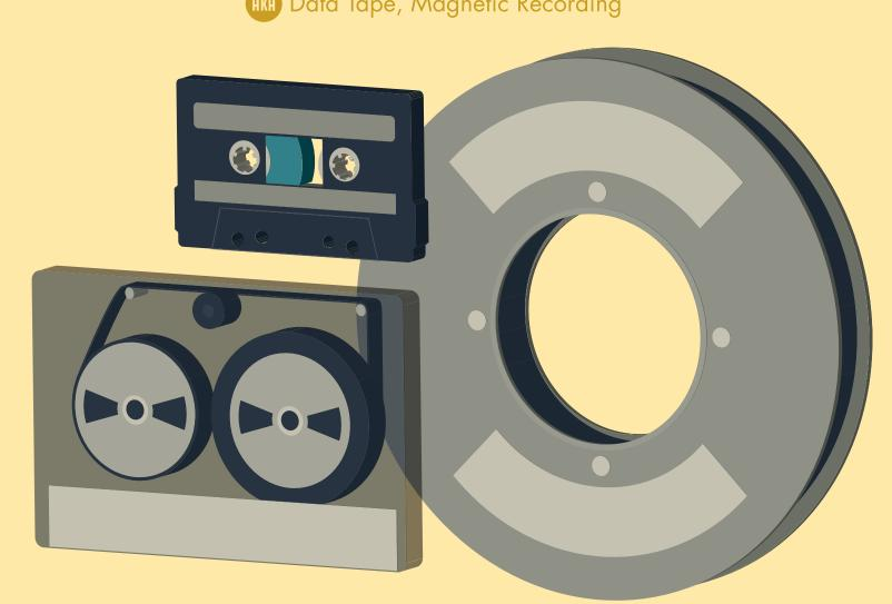
Container Rigid plastic shells or metal reels Variations Cassette, Cartridge, Open reel Capacity Range varies greatly, from MB to TB
